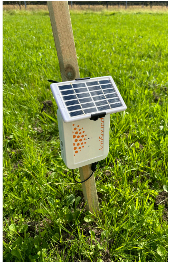
Above: One of the technologies trialled was the 'Polly', an in-field sensor device designed for automated insect monitoring using advanced bioacoustic algorithms to identify passing pollinators.
